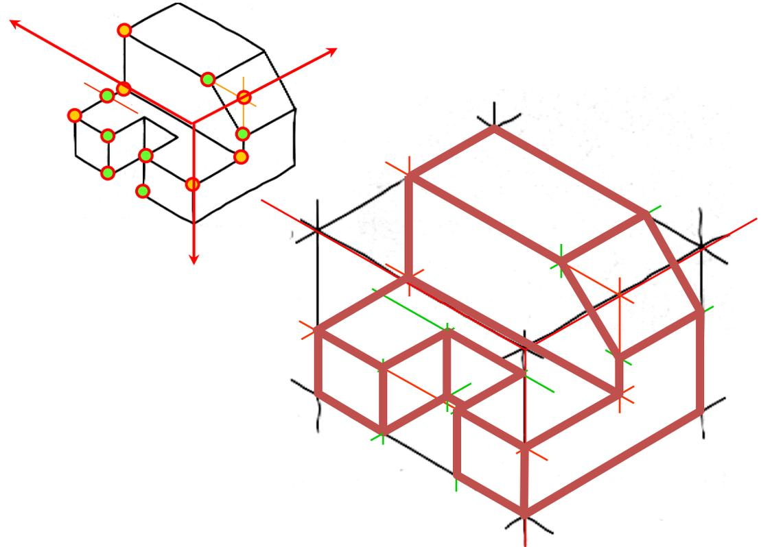
**Note** In isometric sketch/drawing), hidden lines are *omitted* unless they are absolutely necessary to completely describe the object.
