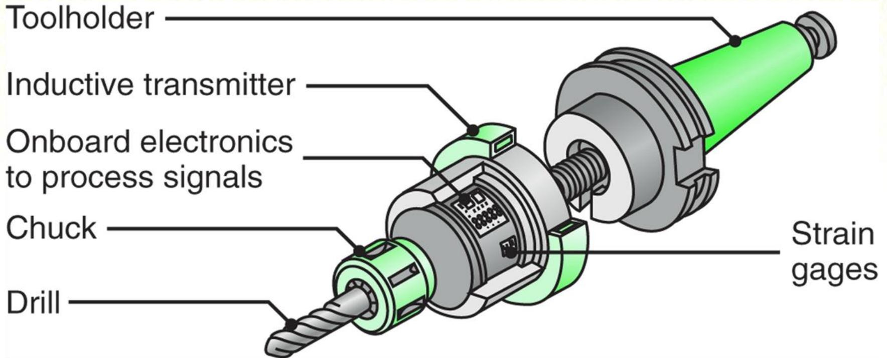
A toolholder equipped with thrust-force and torque sensors (and thus a smart toolholder), capable of continuously monitoring the cutting operation. Such toolholders are necessary for the adaptive control of manufacturing operations.
