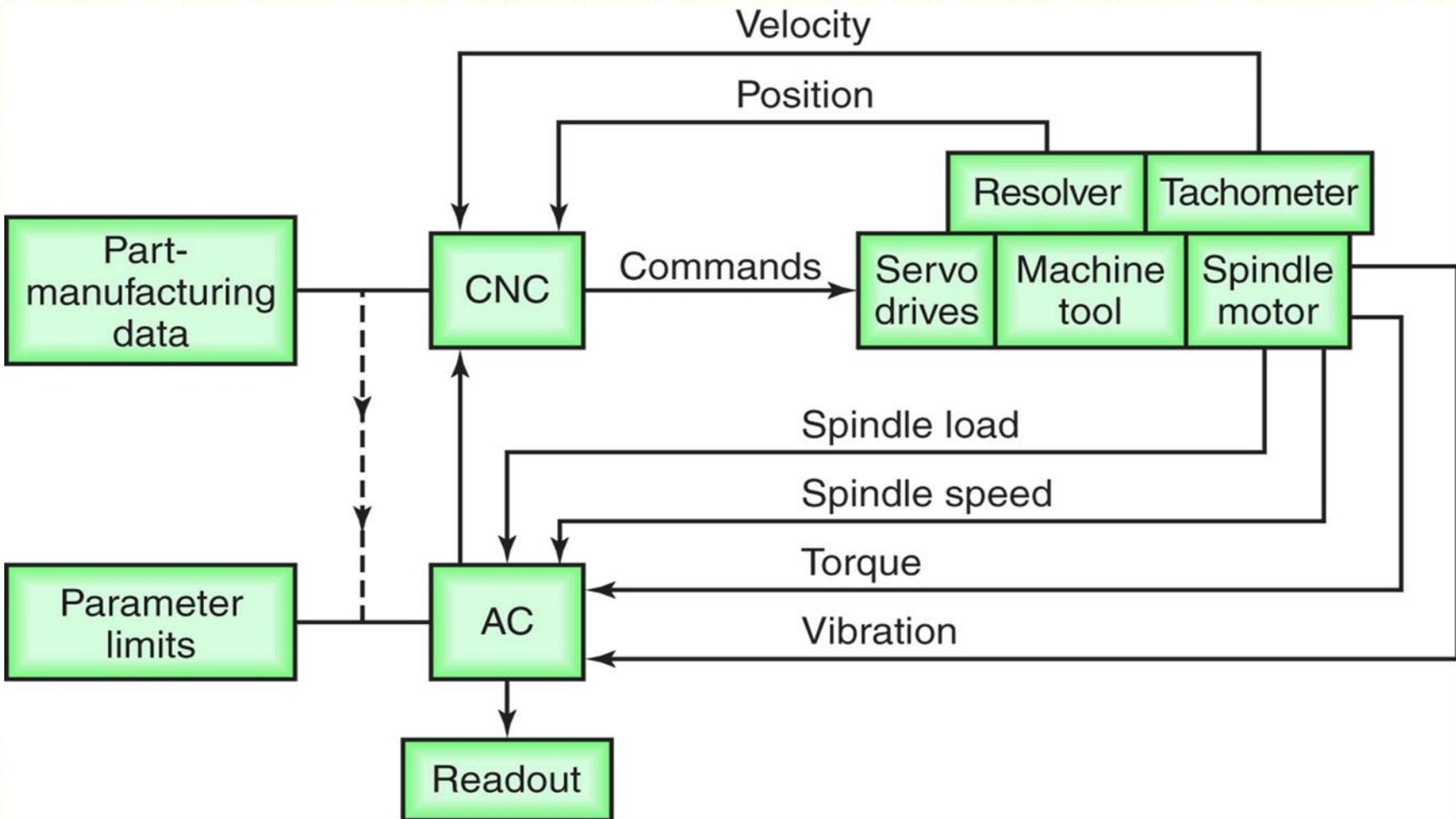
The system monitors such parameters as cutting force, torque, and vibrations. If these parameters are excessive, it modifies process variables (such as feed and depth of cut) to bring the parameters back to acceptable levels.
