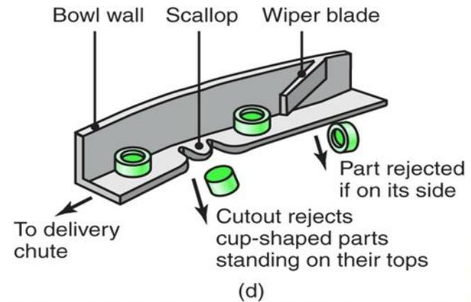
Examples of guides to ensure that parts are properly oriented for automated assembly. *Source: After G. Boothroyd.*
