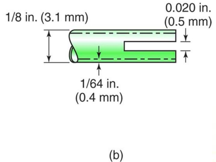
(a) Schematic illustration of for die-sinking applications. (b) Cavities produced by the electrical-discharge machining process, using shaped electrodes. (c) A spiral cavity produced by EDM using a slowly rotating electrode similar to a screw thread. (d) Holes in a fuel-injection nozzle made by EDM; the material is heat-treated steel.
