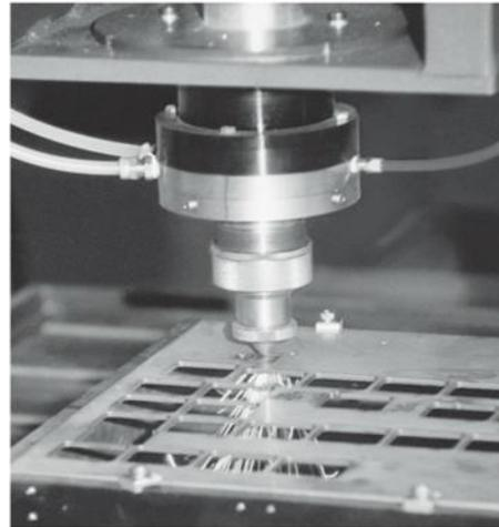
Schematic illustration of the electron-beam machining process. Unlike LBM, this process requires a vacuum, so the work piece size is limited to the size of the vacuum chamber.
