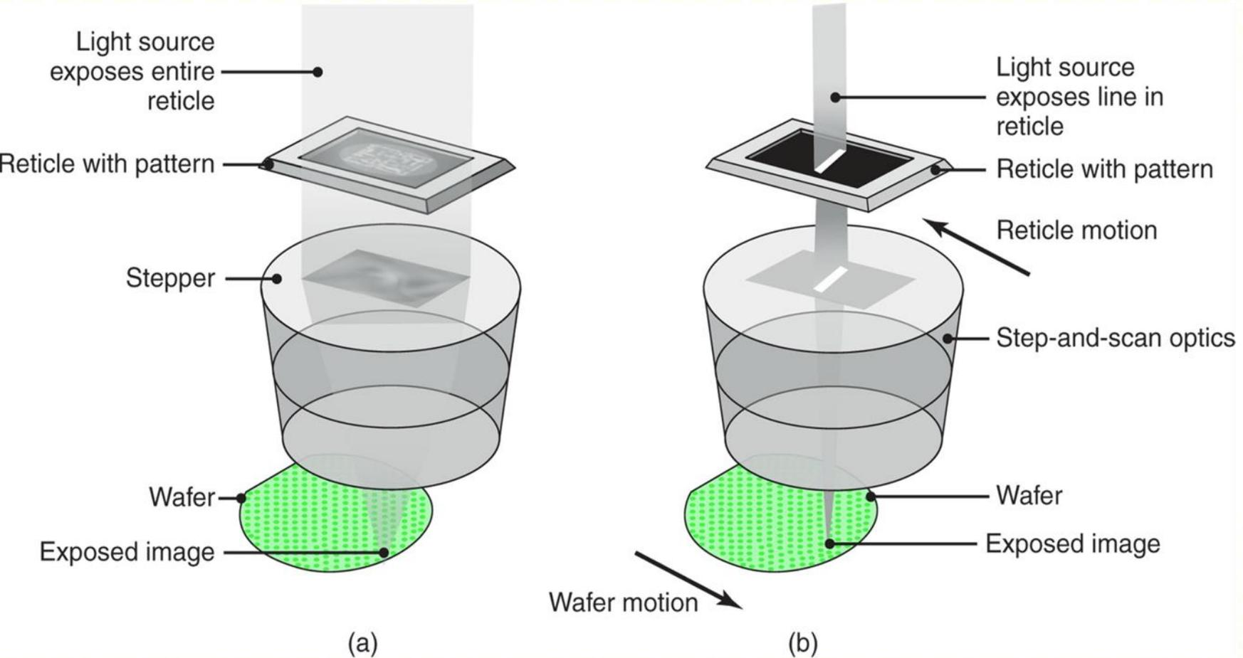
Pattern transfer by photolithography. The mask in Step 3 can be a positive or negative image of the pattern.
