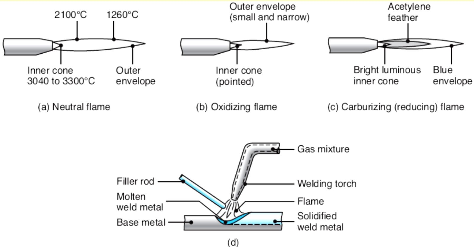
The gas mixture in (a) is basically equal volumes of oxygen and acetylene.
