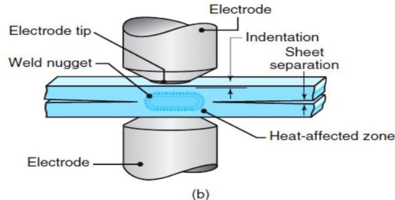
Sequence of events in resistance spot welding. (b) Cross section of a spot weld, showing the weld nugget and the indentation of the electrode on the sheet surfaces. This is one of the most commonly used processes in sheet-metal fabrication and in automotive body assembly.
