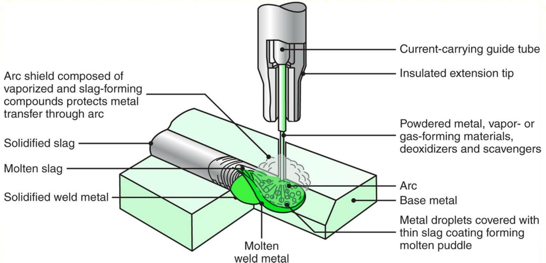
Schematic illustration of the flux-cored arc-welding process. This operation is similar to gas metal-arc welding
