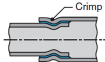
(i) Crimped combination joint
