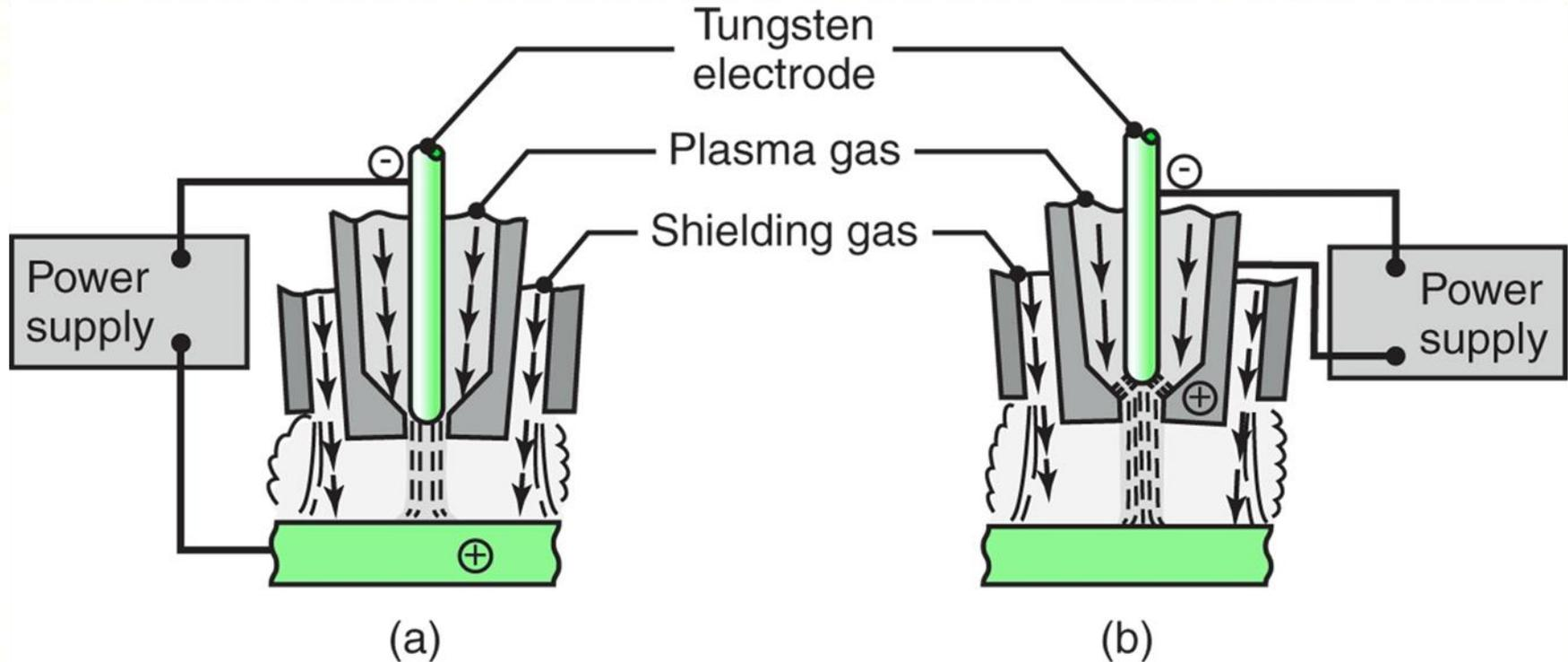
Two types of plasma-arc welding processes: (a) transferred and (b) non-transferred. Deep and narrow welds can be made by these processes at high welding speeds.
