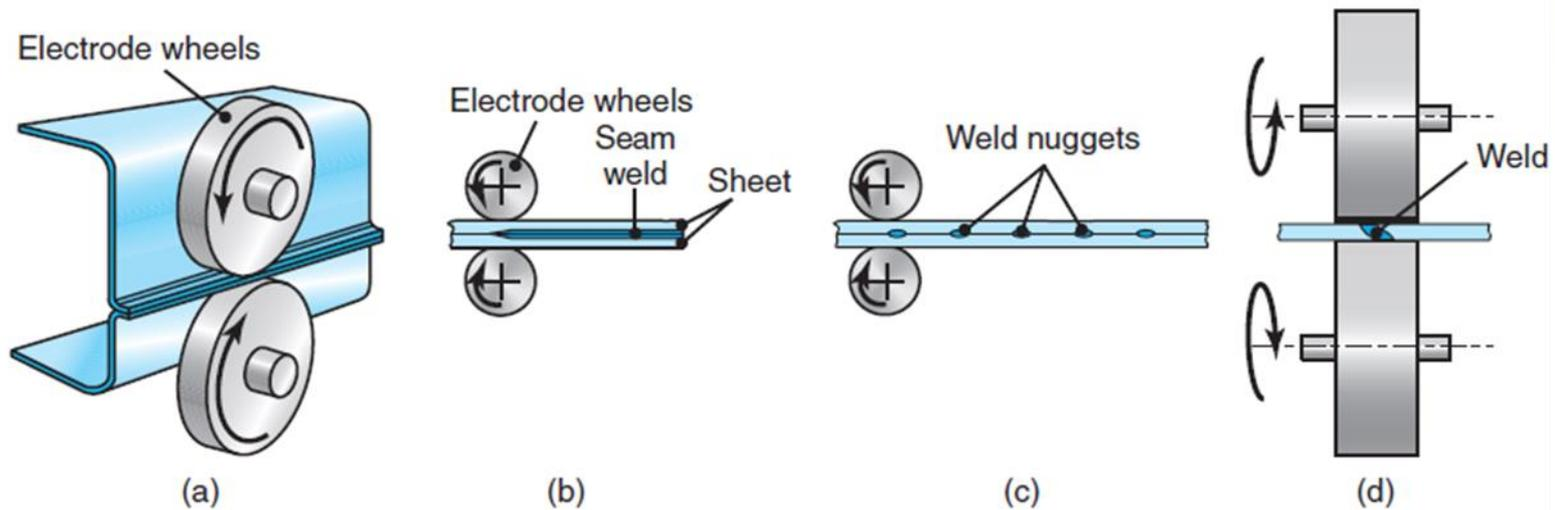
(a) Seam-welding process in which rotating rolls act as electrodes. (b) Overlapping spots in a seam weld. (c) Roll spot welds and (d) Mash seam welding.
