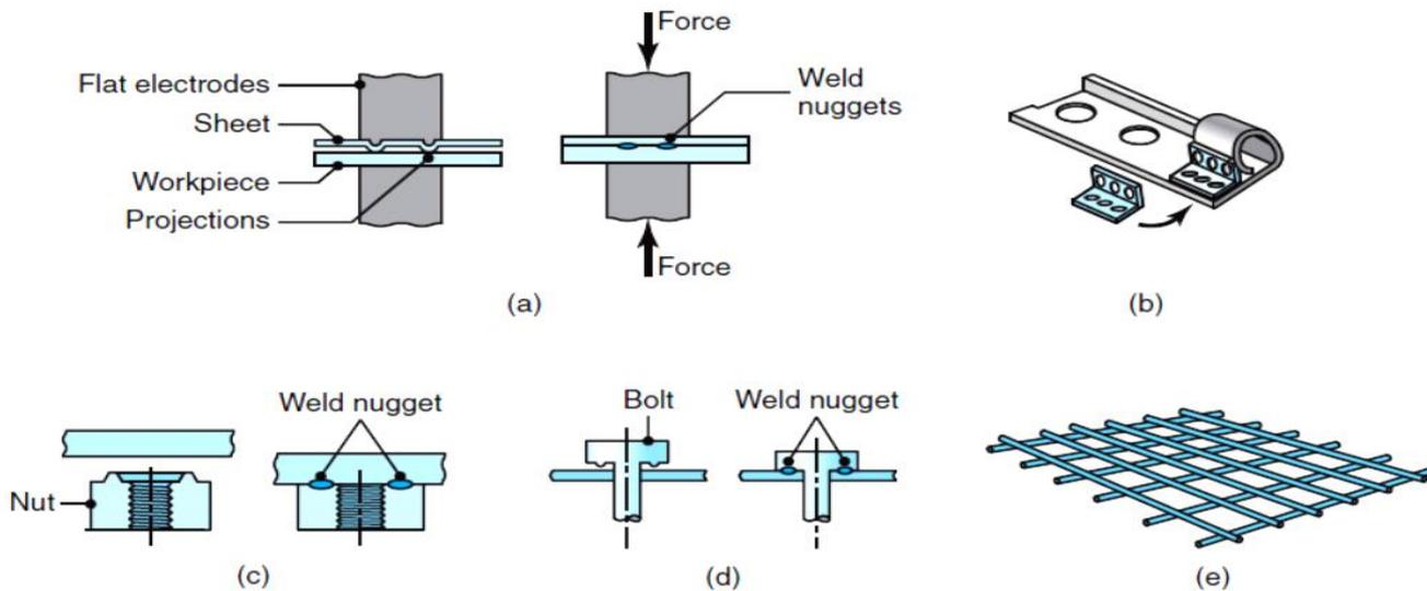
(a) Schematic illustration of resistance projection welding. (b) A welded bracket. (c) and (d) Projection welding of nuts or threaded bosses and studs. (e) Resistance projection welded grills.
