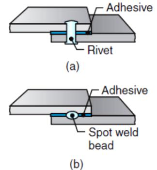
Various joint designs in adhesive bonding. Note that good designs require large contact areas between the members to be joined
