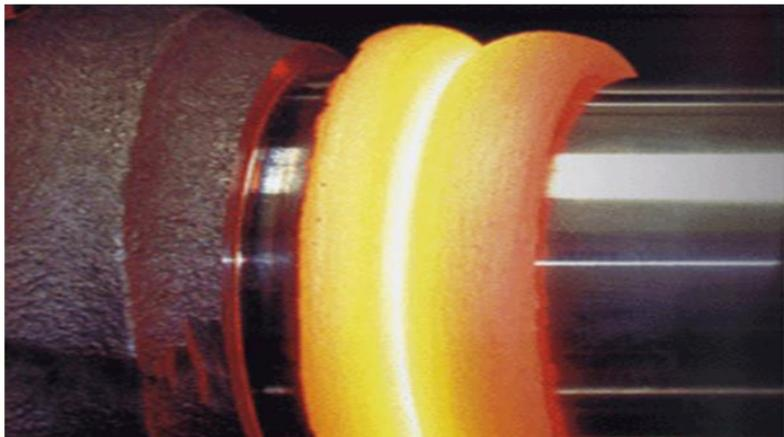
Sequence of operations in the friction-welding process
