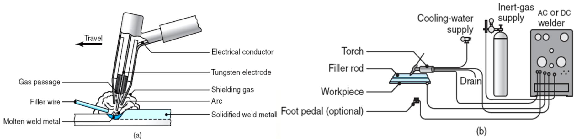
(a) The gas tungsten-arc welding process, formerly known as TIG (for tungsten–inert-gas) welding. (b) Equipment for gas tungsten-arc welding operations.
