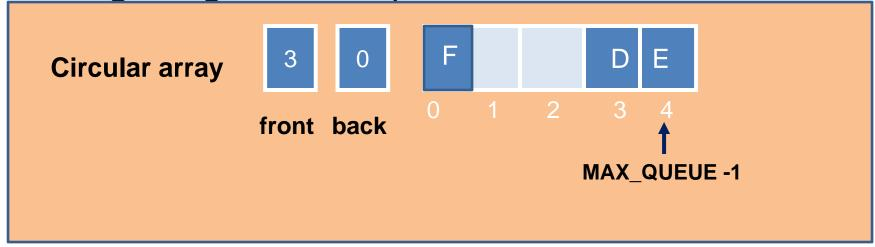
In the figure, to insert F in the queue, F will be inserted at the front queue and restart again at index 0.
