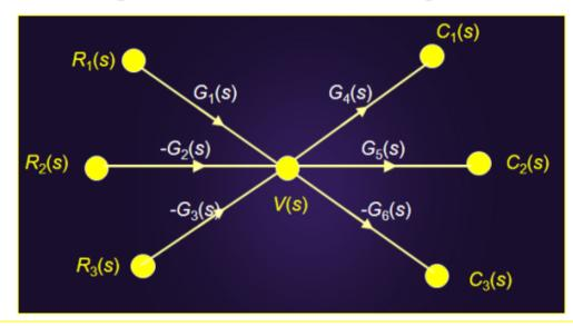
$$V(s) = R_1(s)G_1(s) - R_2(s)G_2(s) - R_3(s)G_3(s)$$
