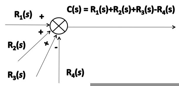
Allows 2 or more signals to be added/subtracted
