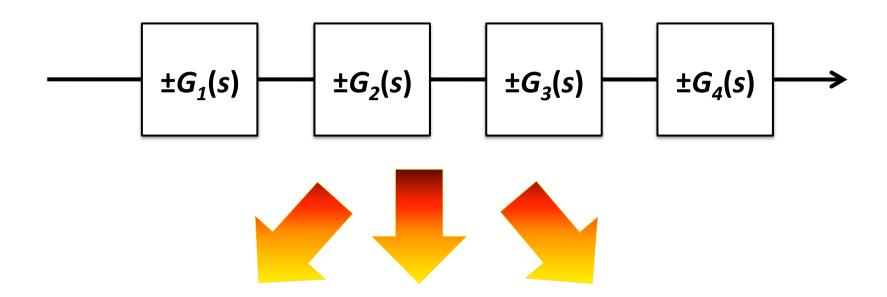
\* The block diagram can be reduced into a single block by multiplying every block to give:
