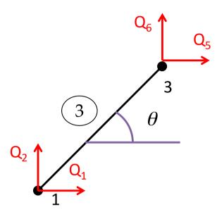
$$\left\{q\right\} = \left(\begin{array}{c} q_1 \\ q_2 \\ q_5 \\ q_6 \end{array}\right)$$
