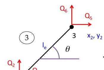
$$\therefore \begin{pmatrix} q'_1 \\ q'_3 \end{pmatrix} = \begin{pmatrix} l & m & 0 & 0 \\ 0 & 0 & l & m \end{pmatrix} \begin{pmatrix} q_1 \\ q_2 \\ q_5 \\ q_6 \end{pmatrix}$$
