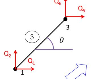
$$\therefore \begin{pmatrix} q'_1 \\ q'_3 \end{pmatrix} = \begin{pmatrix} l & m & 0 & 0 \\ 0 & 0 & l & m \end{pmatrix} \begin{pmatrix} q_1 \\ q_2 \\ q_5 \\ q_6 \end{pmatrix}$$
