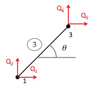
$$\therefore \left( \begin{array}{c} q_1' \\ q_3' \end{array} \right) = \left( \begin{array}{cccc} l & m & 0 & 0 \\ 0 & 0 & l & m \end{array} \right) \left( \begin{array}{c} q_1 \\ q_2 \\ q_5 \\ q_6 \end{array} \right)$$
