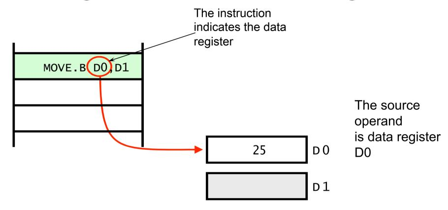
The MOVE.B D0,D1 instruction uses data registers for both source and destination operands
