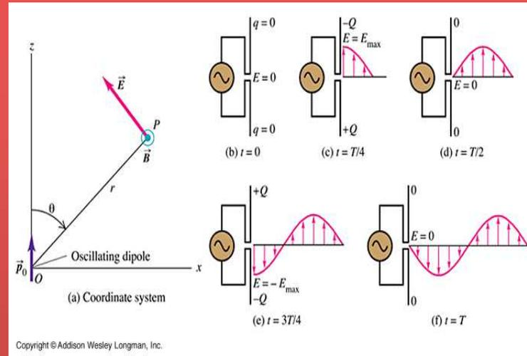
•One cycle in the production of an electro-magnetic wave by an oscillating electric dipole antenna.
