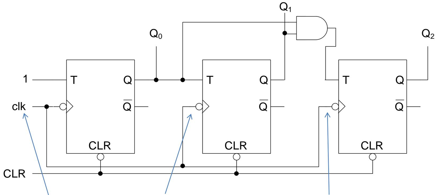
In synchronous counters, a common clk signal is used to clock all flip-flops
