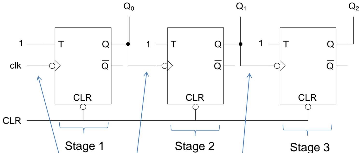
In asynchronous counters, the clk signal is fed to the 1<sup>st</sup> stage only. Subsequent stages take the Q from the previous stage for clk
